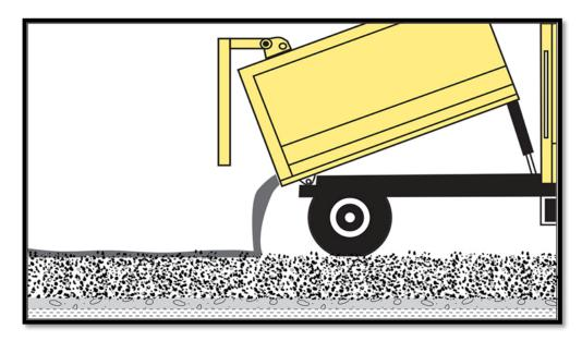
Uniformly spray ENVIROTAC diluted with water. It can sprayed using a Water Tanker with spray bar or emulsion pressure distributor on required surface.
