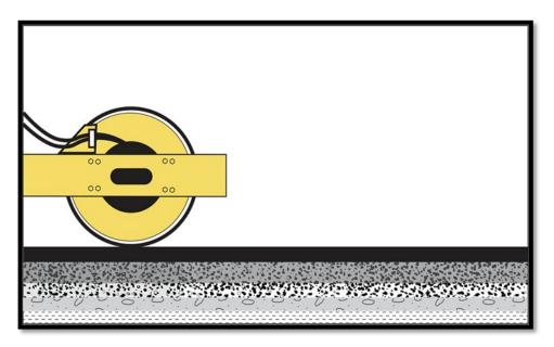
When cured it can be paved with bituminous concrete.
