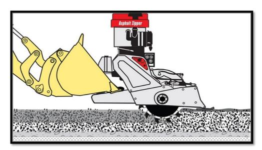
Thoroughly blend material-ENVIROTAC with a predetermined portion of the base/subbase.
