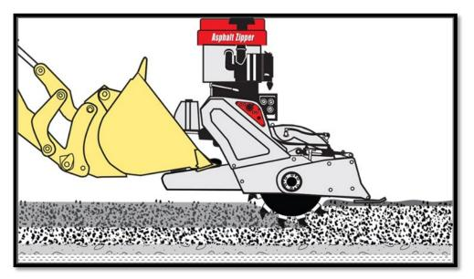
Thoroughly blend materialcement with a predetermined portion of the base/subbase. Hydrate as needed.
