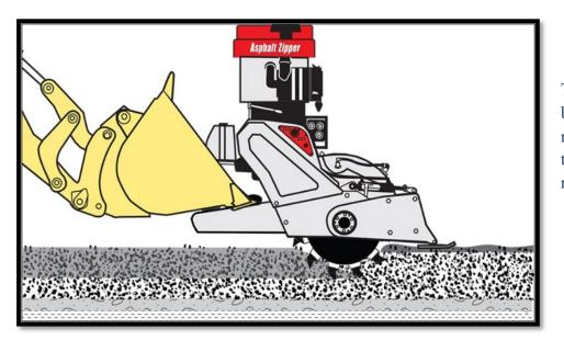
The gravel are laied for the base/sub-base as per the required thickness. Then they are ppulverized the with rototiller/rotavator machine
