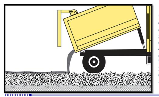
Uniformly spread cement. Cement can be spread by a cement spreader or markings can be made and cement bags can be open directly on the base or subbase. Cement can also be mixed in the batching plant along with soilaggregate mixture and then aid with a paver.
